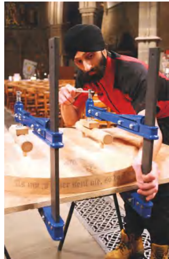
▲ Pic.22 Clamping the handles into position
